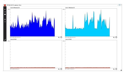
The RTX64 2013 Latency View tool provides users the ability to view and compare system timer response latencies on multiple cores at the same time. Users can also add loads to stress the system to determine if it can meet their application's real-time needs.
